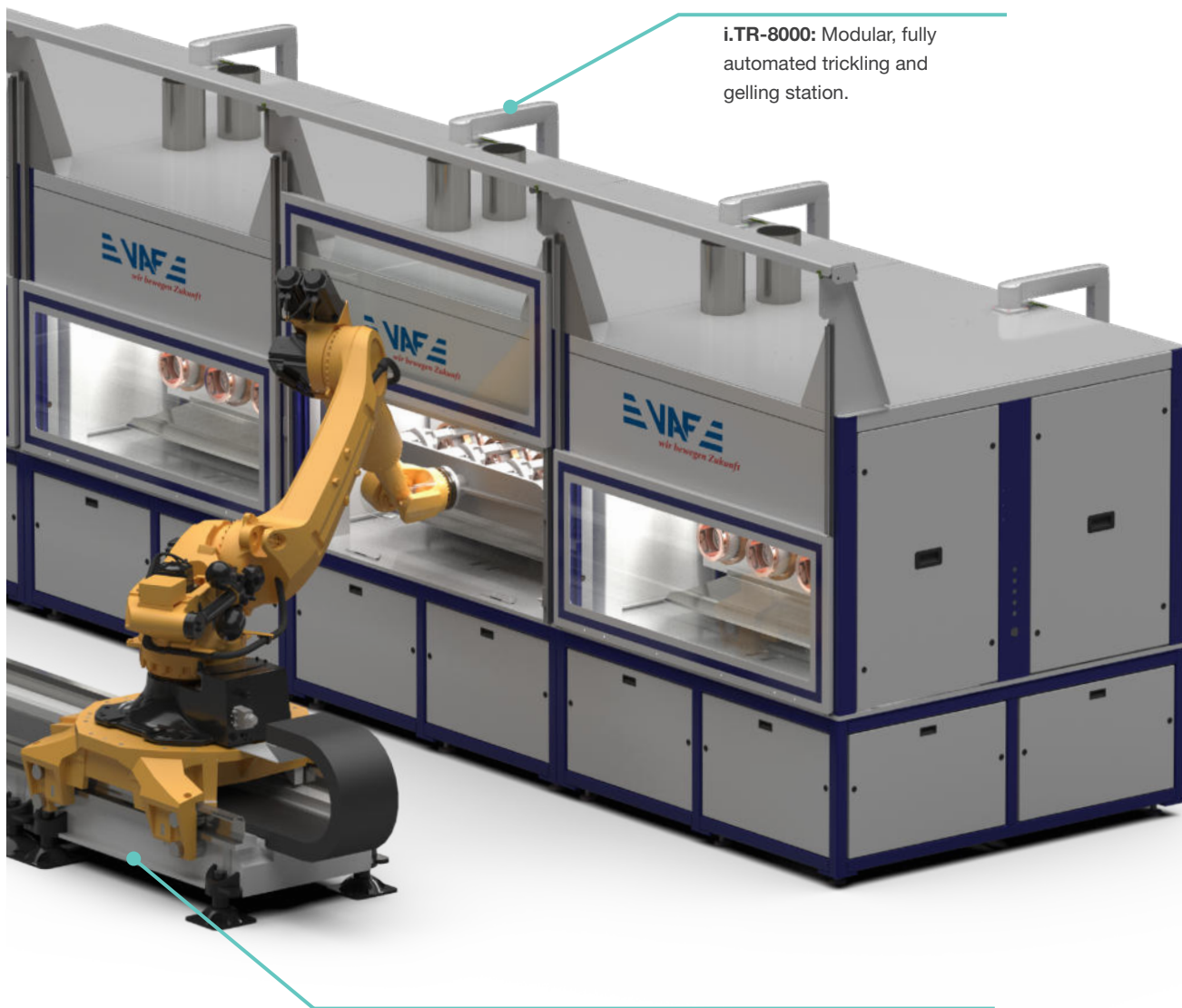
7-axis robot: Loading of preheated components, unloading of dribbled and gelled components. Alternatively, other loading concepts can be implemented.
